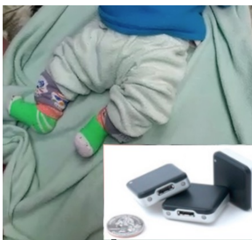
Figure 1. Infant wearing sensors on each ankle, in pockets of ankle bands. Inset shows 3 sensors (APDM, Inc.) with a United States quarter for reference.
